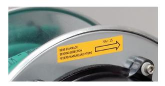
The spring reels not equipped with a roller guide arm are delivered without pre-tension set-up. In this case, prior to use, the spring motor must be pre-tensioned with the appropriate number of turns 'NA' and direction as indicated on the drum flange.
