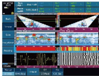
Real-time coupling monitoring for PA long pipe solution.
