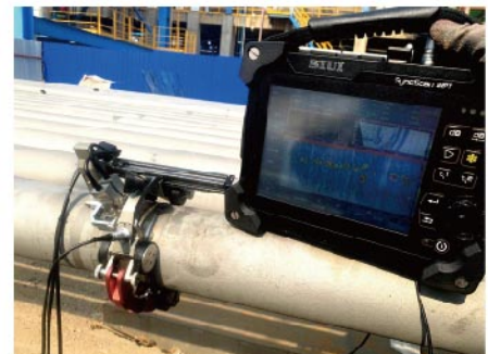
Austenitic weld inspection
