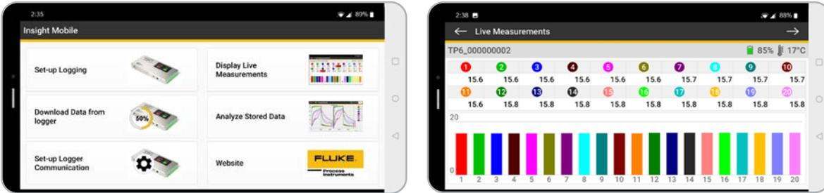
Our Insight™ for Mobile software allows you to reset, download, and analyze thermocouple operation on your tablet or smartphone via Bluetooth connection.
